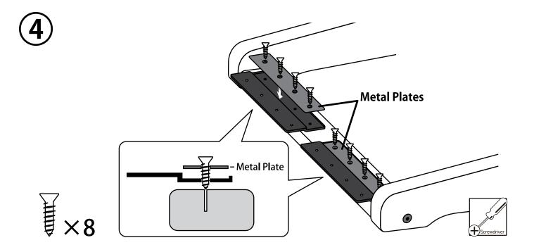
Locate the metal cover plates into the polyurethane hinges. Then attach the hinges to the treadle rail with 16mm (5/8") screws.
