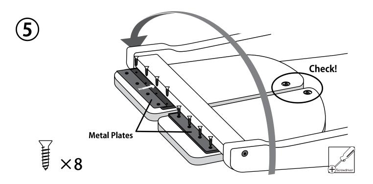
Lay the base on its back. Locate the metal cover plates into the polyurethane hinges. Then attach the treadle boards to the hinges with 16mm (5/8") screws.
