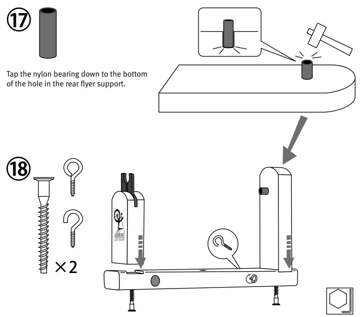
Secure the front and back flyer supports to the maiden bar with 50mm (2") Allen head screws. Screw the hook and eye into the maiden bar.
