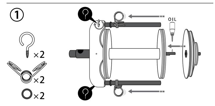
Thread 2 hooks into the flyer base. Slide the 2 rubber O-rings onto the flyer arms Squeeze and slide the yarn guides onto the flyer arms Apply a drop of oil to the flyer shaft and slide the bobbin and flyer whorl into position.
