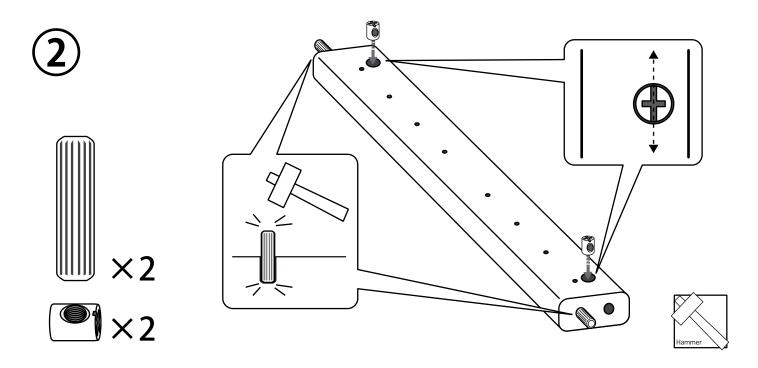
Tap wooden dowels to the bottom of the holes in either end of the treadle rail.
