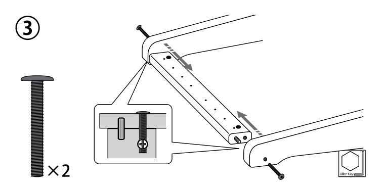
Loosely attach the feet to the treadle rail with 50mm (2") bolts and barrel nuts. Sit the base on a flat surface and check the feet are level. Then tighten the bolts.
