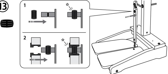
Slide the inner shell of the conrod universal joint onto the crank until it clicks into the groove. Then click the front conrod onto the universal joint on the crank.
