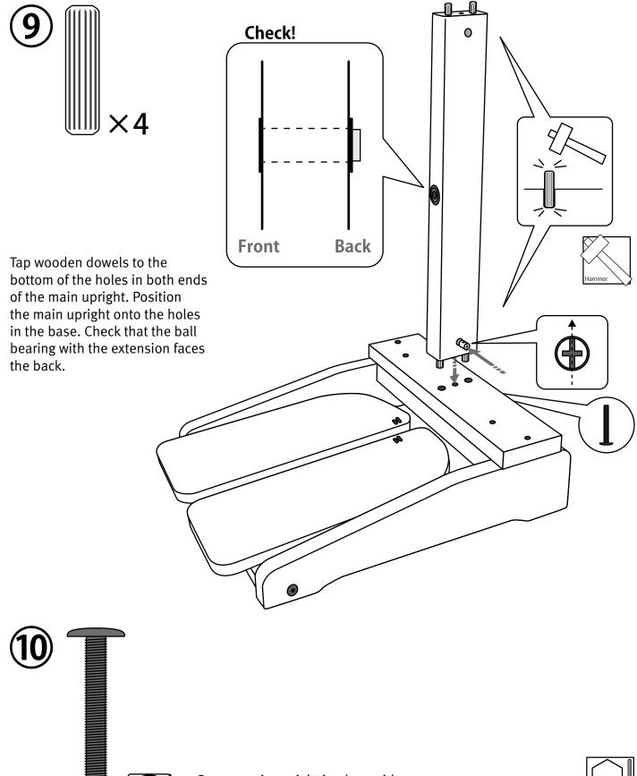
Secure main upright in place with a 50mm (2") bolt and barrel nut.
