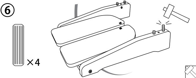
Turn the base back over. Tap wooden dowels down to the bottom of the holes in the feet.
